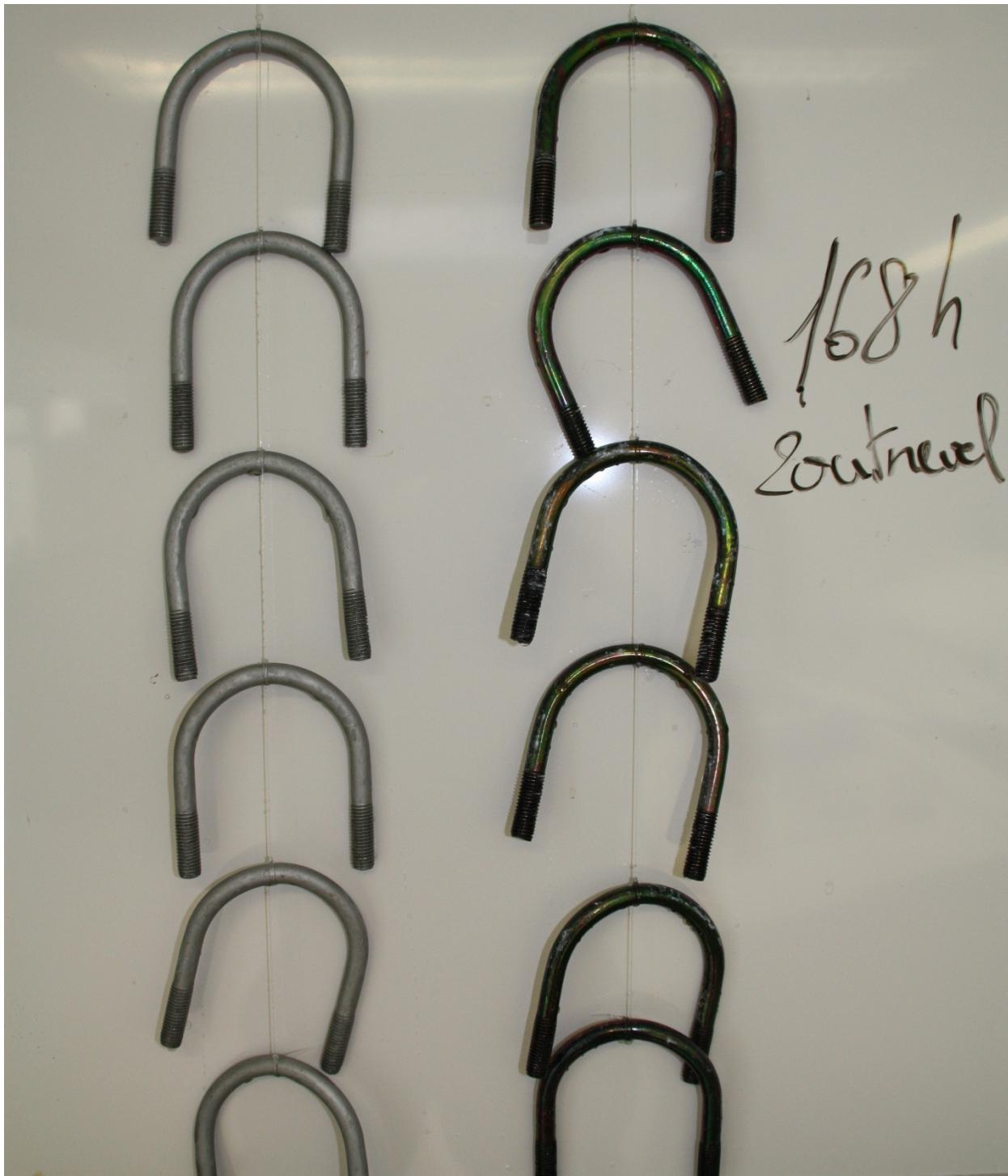
Salt Spray Test NEN EN ISO 9227 NSS after **168 hours**
