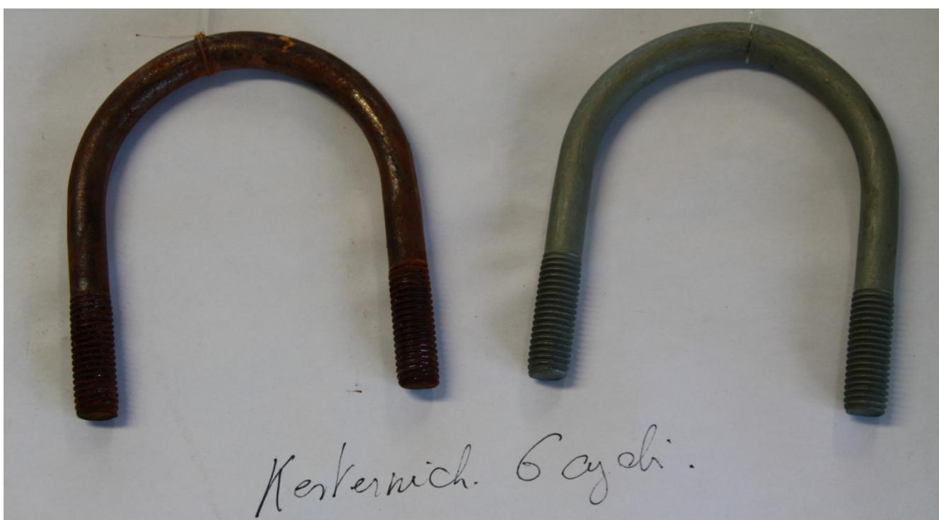
Kesternichtest NEN EN ISO 3231 SWF 2,0L after 6 rounds. Blank steel appears on Zincrolyte<sup>®</sup> treated part.
