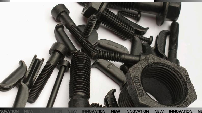
Deltacoll® Black is an intense black surface treatment with high corrosion resistance and low coating thickness. It consists of a black passivated electrolytic zinc layer coated with an inorganic black topcoat containing silicate and titanium and providing the uniform black shiny look. Because of the limited layer thickness and integrated lubricant, Deltacoll® Black is an ideal solution for (small) parts where tolerance is limited, such as screws, bolts, nuts, etc.
